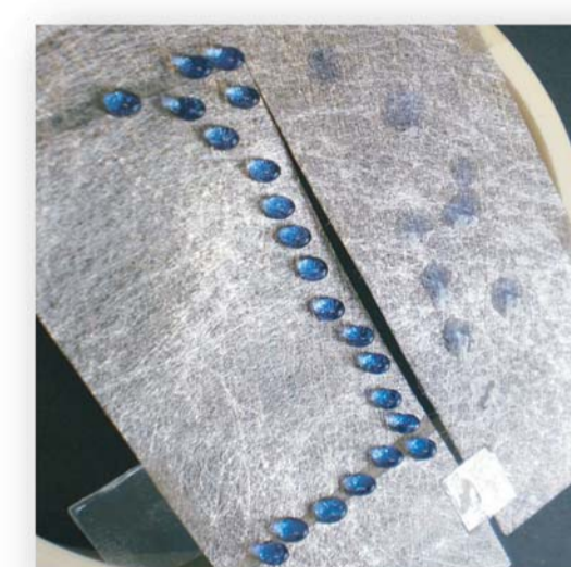
Figure 8: Metalized (aluminum coated) polyester nonwoven. Left: hydrophobic plasma topcoating, right: hydrophilic plasma topcoating. Ink droplets show the specific surface functionalization.
